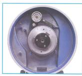
The self adjusting belt tension spring is designed for smooth, quiet and trouble-free operation.
